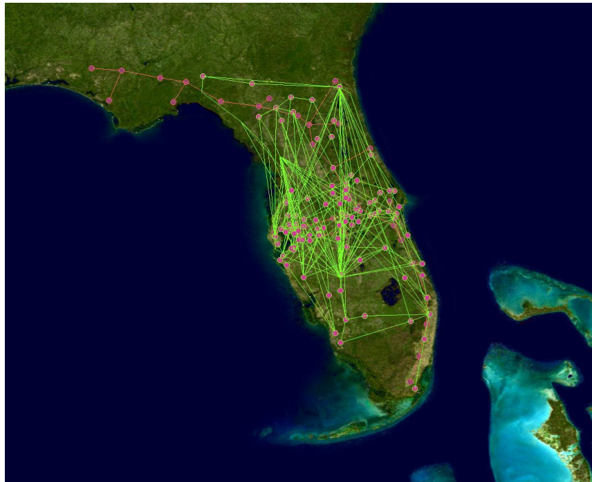
Figure 4-11 – Sample Florida State Electric Power and Natural Gas Components as overlays on a Satellite Picture provided by NASA OnEarth WMS Server. Electric power components are connected with green, natural gas components are connected with red lines.
