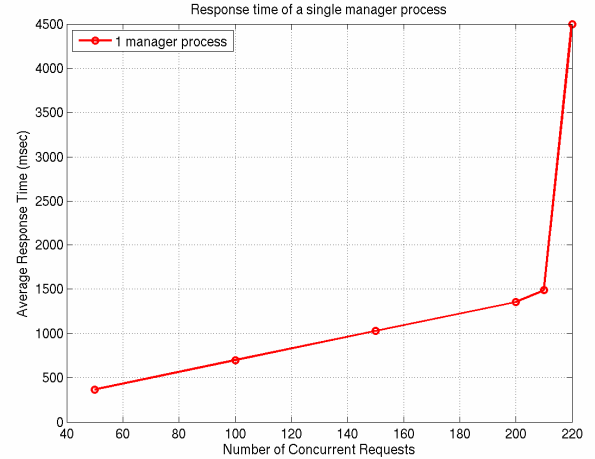
Figure 8 Saturation point for a single manager
