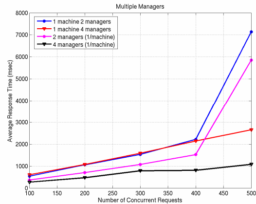
Figure 6 Response time comparison (Increasing manager processes on same vs. multiple machines)
