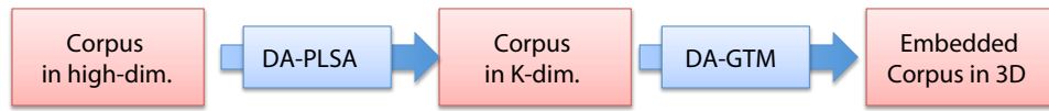
Figure 14: A workflow to visualize large and high-dimensional document corpus in a virtual 3-dimensional space. A high-dimensional document corpus will be processed by DA-PLSA to reduce the original dimension to an arbitrary smaller dimension, then, followed by DA-GTM to compute an optimal embedding in a 3-dimensional space.
