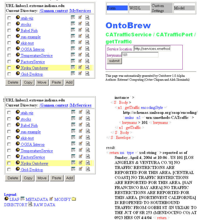
Figure 6. The Xydra-Ontobrew service. The directory service contains a link to the Xydra. Xydra then requests a URL for the WSDL for a service. The supplied url, http://www.xmethods.net/sd/2001/CATrafficService.wsdl, is the location of the WSDL for web service for the California Highway Traffic Condition reporter web service. Ontobrew dynamically generated the
