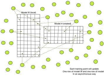
Asynchronous: Random access to model data Good for thread-level workload balance.
