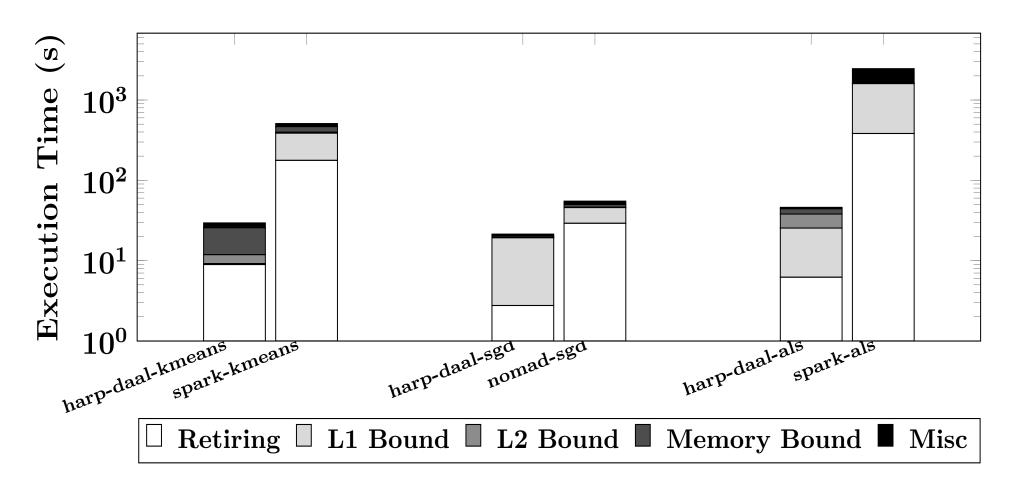
Spark-Kmeans and Spark-ALS dominated by Computation (retiring), no AVX-512 to reduce retiring Instructions, Harp-DAAL improves L1 cache bandwidth utilization due to AVX-512
