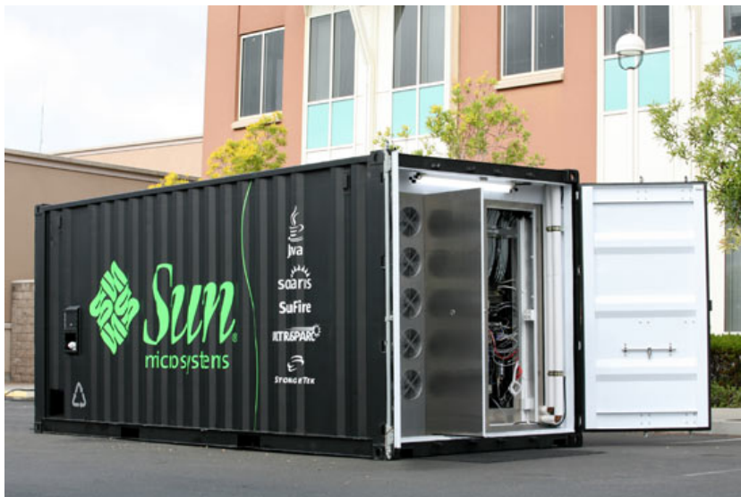
FIGURE 1.9: Sun Modular Datacenter
