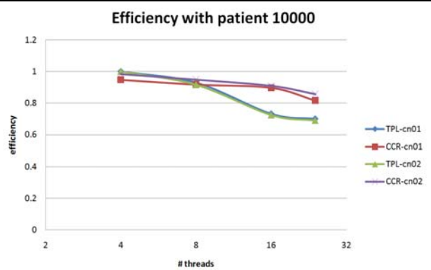
Fig. 20. Parallel Efficiency comparing CCR and TPL for Multi-Dimensional Scaling using 10,000 pt patient data on 24 core Intel and AMD machines
