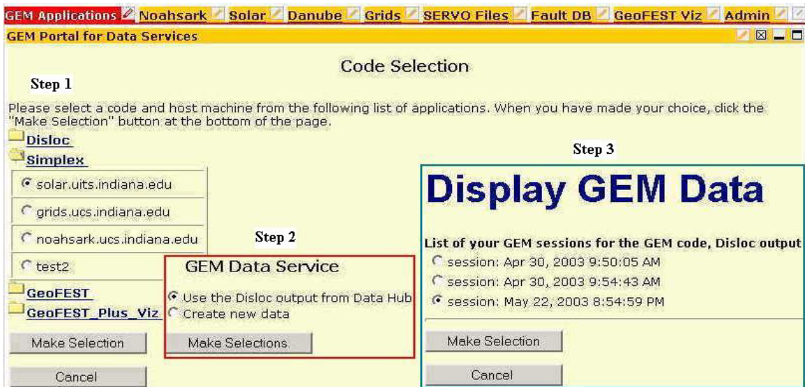
Figure 7.7: Selecting a GEM code for simulating and a host for running (Step 1), input data format which is used for the code (Step 2) and displaying the GEM data in user’s session (Step 3).
