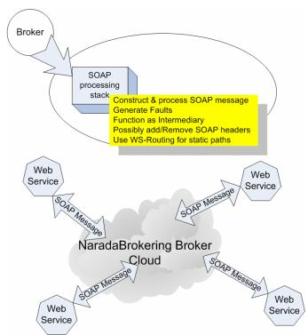
Figure 12: Web Services interacting with the substrate
