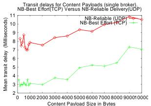
Figure 5: Transit Delay comparison (single broker)
