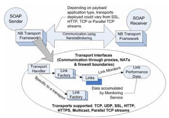
Figure 11: Incorporating support for SOAP in the transport layer
