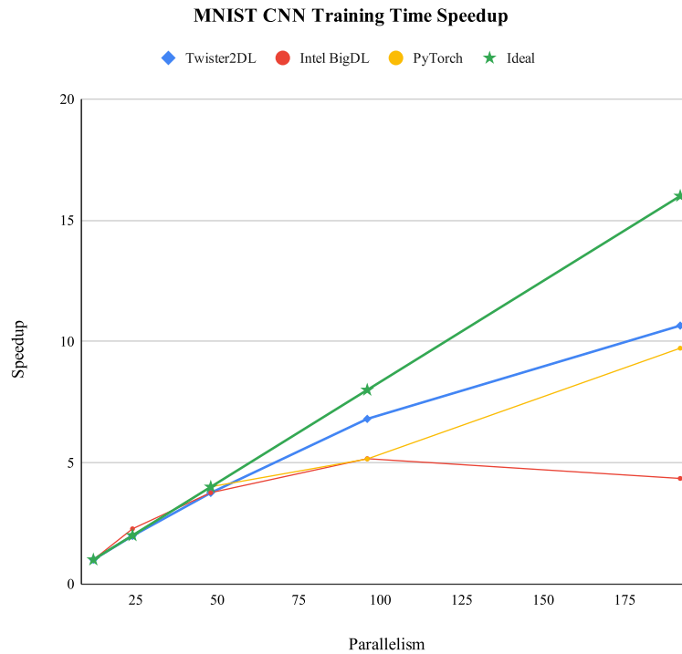
Figure 5.13: Speedup achieved by frameworks compared to Ideal speedup for MNIST CNN training
